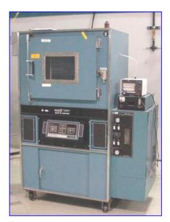
Additionally *iEL* has ten environmental chambers separate from the laboratory that are used for non-fuel applications. Capabilities include: Thermal Cycle, Two High Rate of Change, Three Zone Thermal Shock Chambers, Liquid Thermal Shock, Ozone and Humidity.
